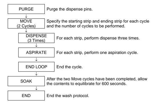
Figure 9. Example of a Wash Protocol
